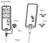
Please stop turning while the key applied to the knob rotates about  $45^\circ$ , otherwise, the key will be damaged : the same situation in the opposite direction. Fig. 3. is a reference angle.  $90^\circ$
