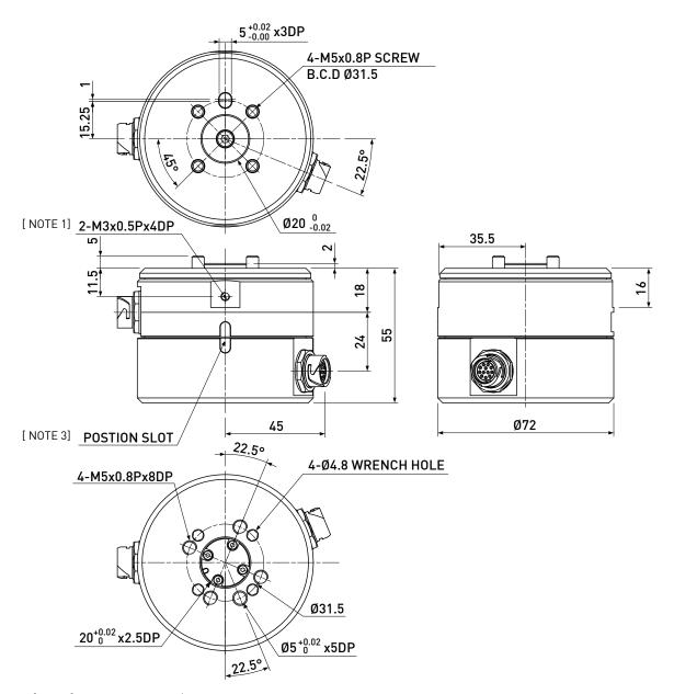
[Note 1] If the HIWIN RA605/RT605 robot manipulator accessory kit is not attached, please make a fastener in accordance with the aligning slot in the above drawings and install it on the stationary part of driving source, in order to prevent the rotation of stator part of rotary joint.
