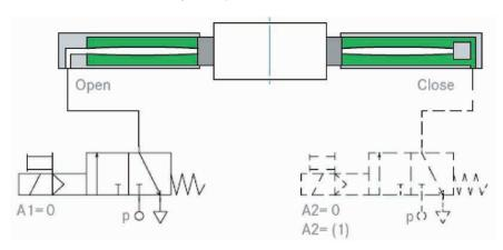
Fig. 3.6 Pneumatic connection of the parking brake
