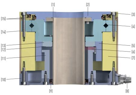
Fig. 3.1 Main components of a rotary table
